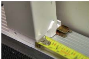
5a: Guide rail measuring. In this example, the guide rails will be 34 5/8" (34 1/2" + 1/8")
